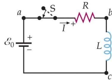
O) An inductance  $L$  and resistance  $R$  are connected in series with a battery, as shown above. A long time after the switch is closed, the current is 2.5 A. when the battery is switched out of the circuit by opening the switch and simultaneously connecting the left side of the resistor to point  $c$ , the current drops to 1.5 A in 45 ms.
