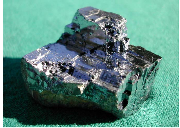
Figure 1.5 CUBIC CLEAVAGE - Three directions @ 90^\circ .
