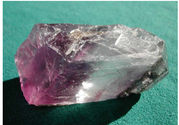
Figure 1.7 OCTAHEDRAL CLEAVAGE - Four directions parallel to the sides of an octahedron.
