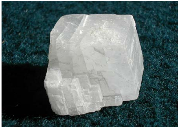
Figure 1.6 RHOMBOHEDRAL CLEAVAGE - Three directions parallel to the sides of a rhombohedron.
