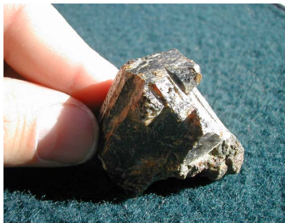
Figure 1.8 DODECAHEDRAL CLEAVAGE – Six directions parallel to the sides of a dodecahedron.
