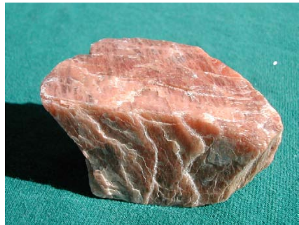
Figure 1.3 – PRISMATIC CLEAVAGE – Two directions @ ~90°.
