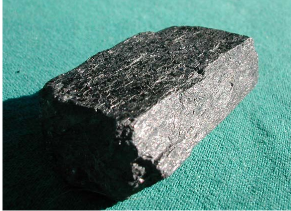
Figure 1.4 PRISMATIC CLEAVAGE – Two directions @ \sim 57^\circ and 123^\circ .
